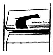
2. Lift the signal arm so it clicks into the OFF (up) position. Ice can still be dispensed, but no more can be made.
